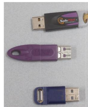
Figure 1 - USB Security Keys used by AcornPipe
